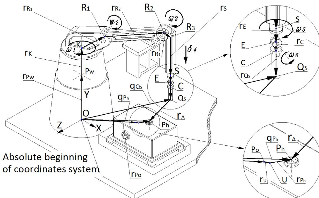
Fig. 2. Location of the assembly system components
