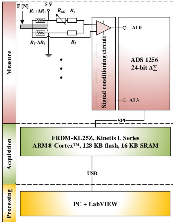
Fig. 1. Functional blocks of the measurement system
