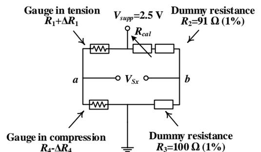
Fig. 4. Wheatstone's bridge circuit applied in the measurement sensor
