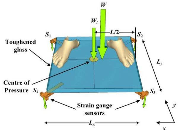
Fig. 3. General view of the platform with forces, sensors  $S_1, S_2, S_3, S_4$  and coordinates assignment
