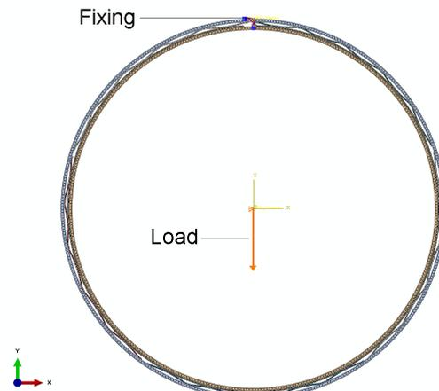
**Fig. 2.** FEM model with fixing and load
