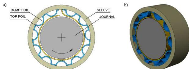
Fig. 1. Basic parts of a foil bearing
