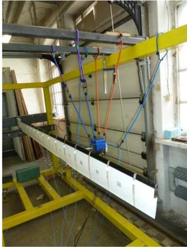
**Fig. 1.** Blade mounted in a test stand
