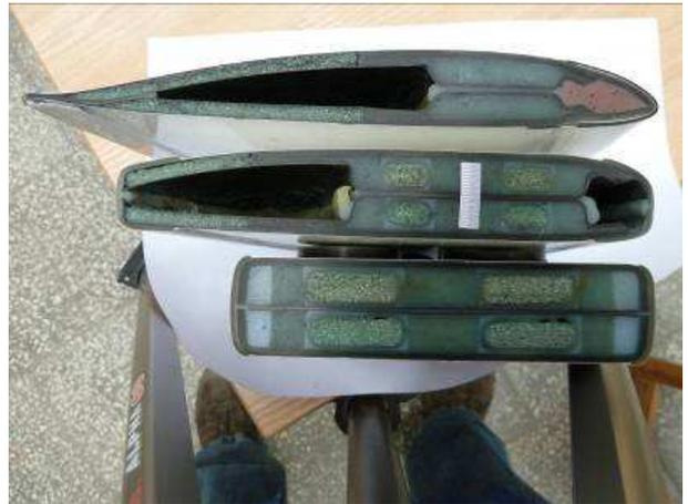
**Fig. 6.** Cross-section of a composite blade
