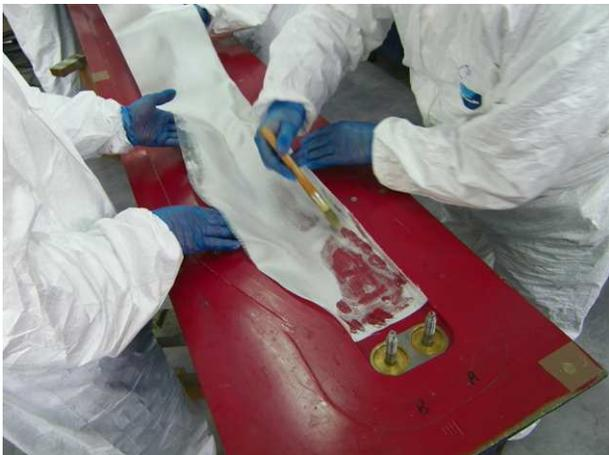
**Fig. 3.** Mould with fiber composite
