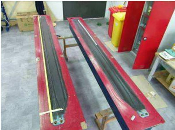
**Fig. 2.** Moulds of blade
