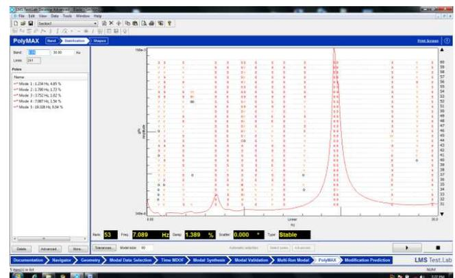
Fig. 11. Stabilization diagram obtained by LMS PolyMAX method
