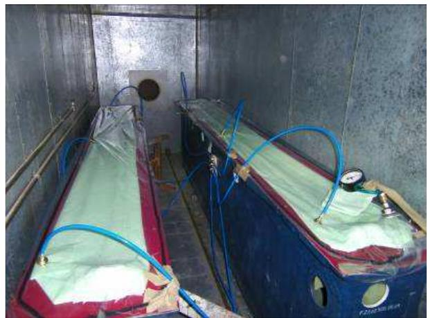
**Fig. 5.** Upper and lower halves of a blade part in oven
