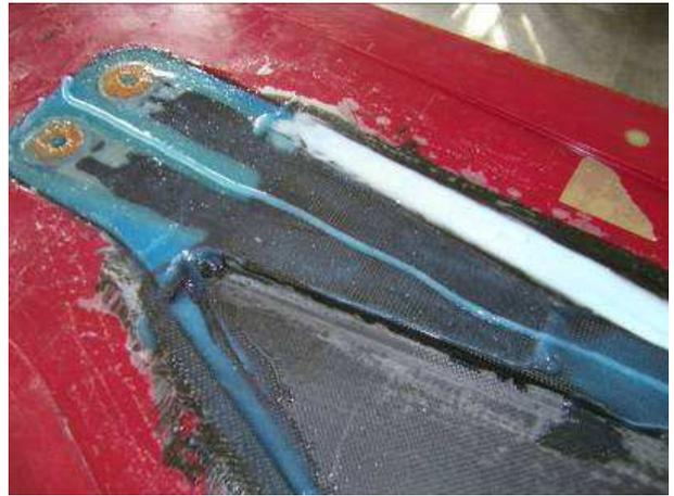
**Fig. 4.** Mould with roving and carbon composite
