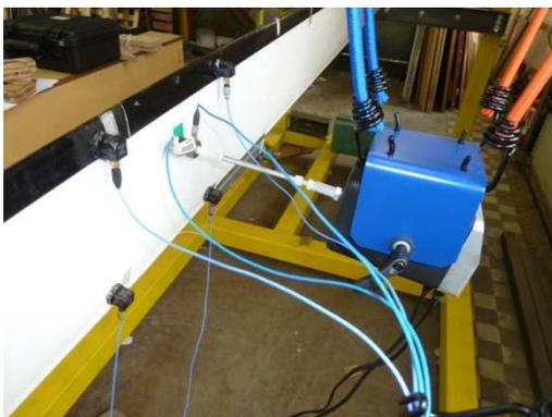
Fig. 8. Vibration test setup of a blade from main rotor of the IS-2 helicopter
