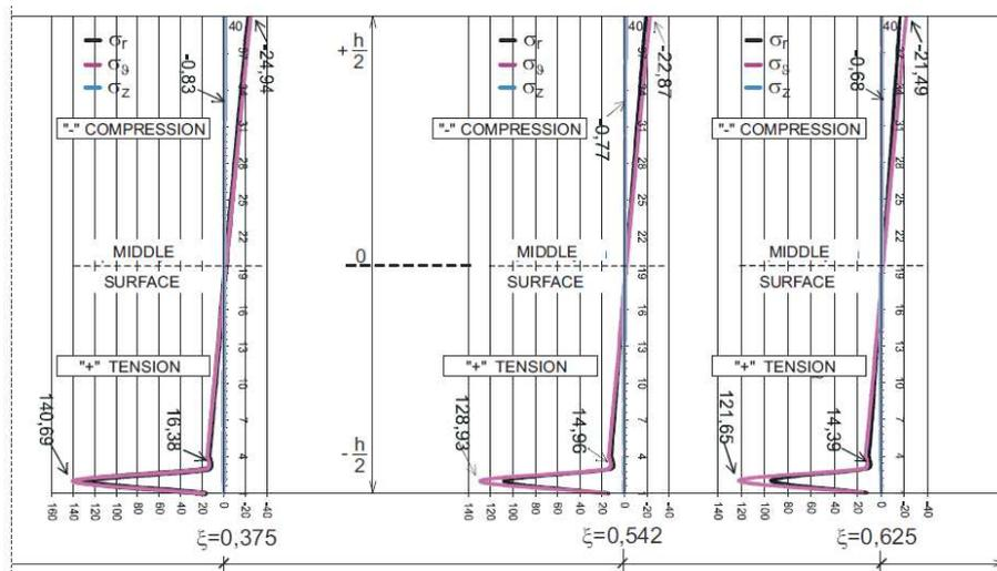
Fig. 7. Stress analysis results  $\sigma_r(\xi), \sigma_\nu(\xi), \sigma_z(\xi)$  in the parameter structure (4) with  $j = 2$
