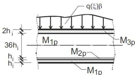
Fig. 8. Crosswise heterogeneous slab with  $j = 3$
