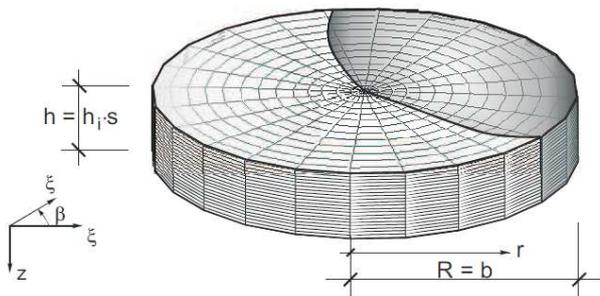
Fig. 3. Discrete model of a circular slab
