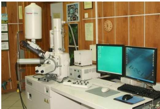
Fig. 1. Scanning electron microscope Hitachi S-3000N
