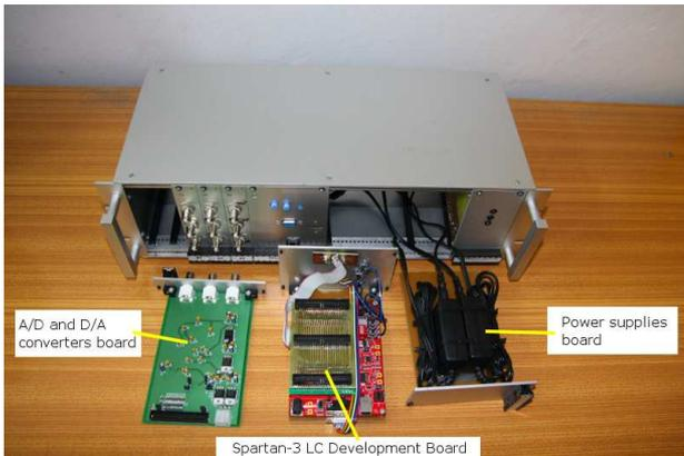
Fig. 2. Active magnetic bearings controller hardware
