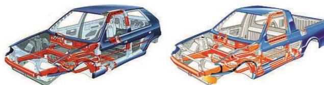
Fig. 1. Reinforcement of the frame with the crumple zone (Szkielet, 2017)
