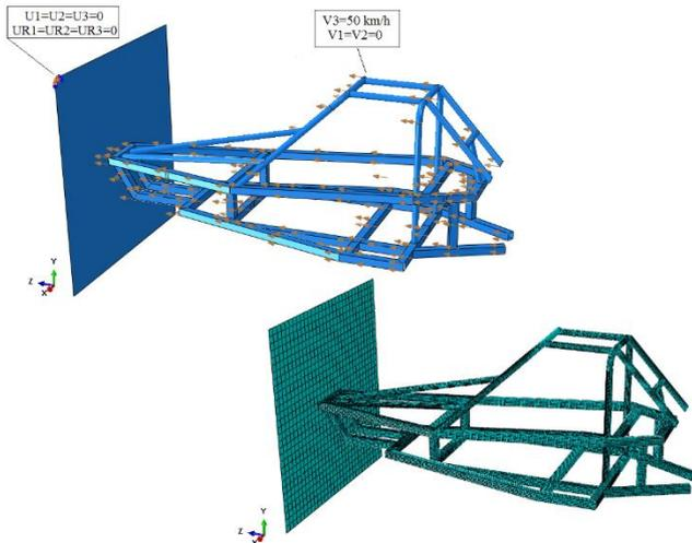
Fig. 6. Boundary conditions and discrete model
