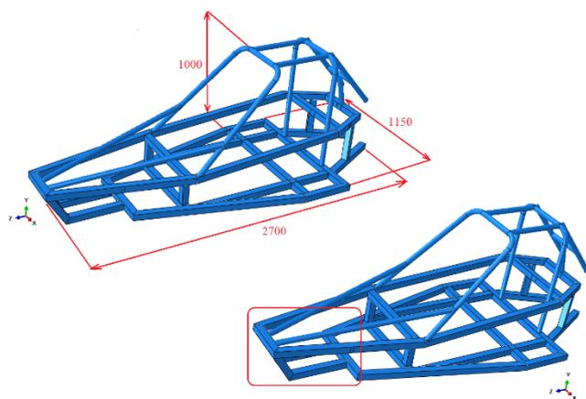
**Fig. 3.** Geometrical parameters of the model and crumple zone
