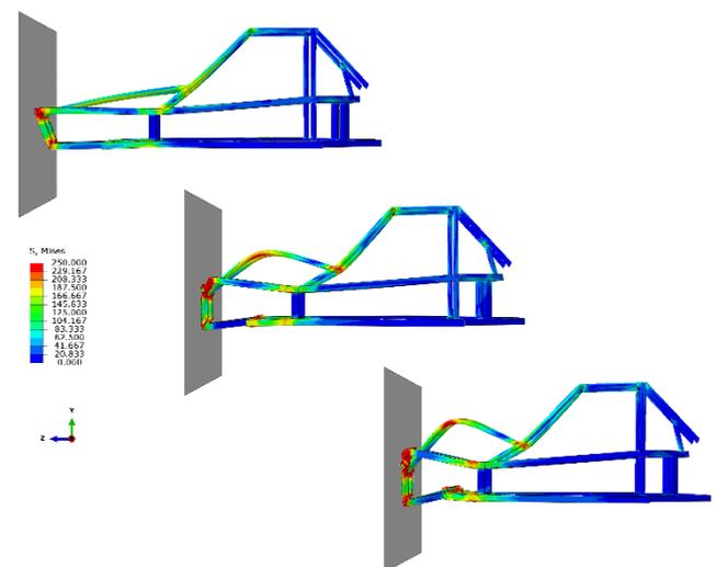
Fig. 8. The frame damage in 0.0045 s, 0.0225 s and 0.045 s
