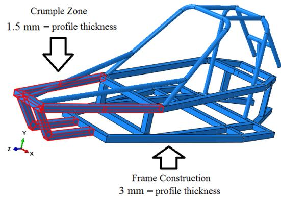
**Fig. 4.** Frame construction detailing areas
