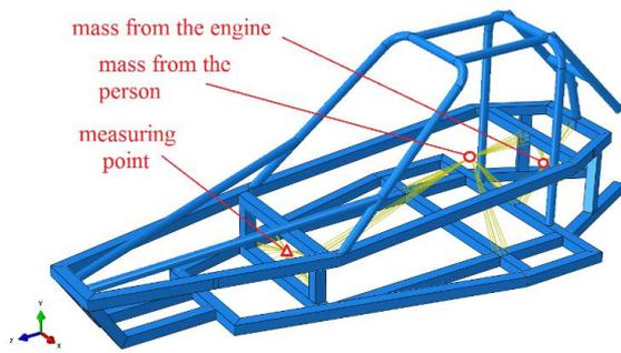
Fig. 5. The frame structure with the included loads from the engine and the person together with the presented measuring point
