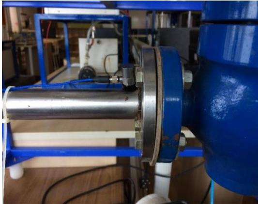
Fig. 5. Mounting of Accelerometer
