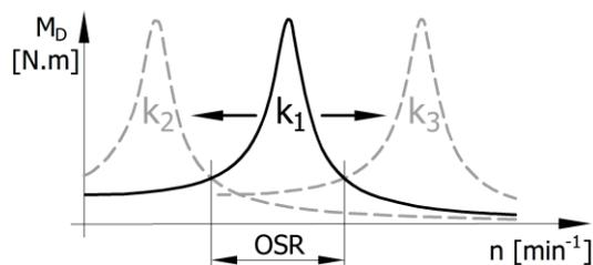
Fig. 1. Mechanical system tuning principle
