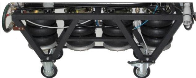
Fig. 3. The mobile platform with 4 air springs Rubena 340/3
