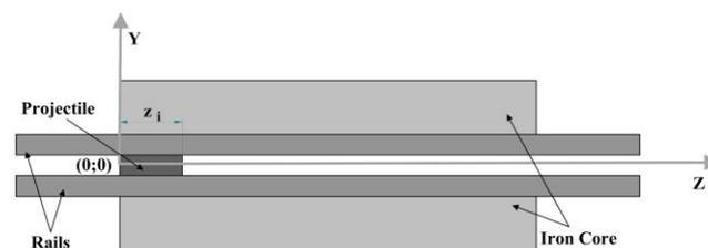
Fig. 6. Initial position of the projectile
