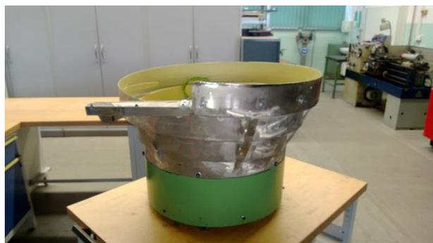
Fig. 1 Bowl feeder for testing
