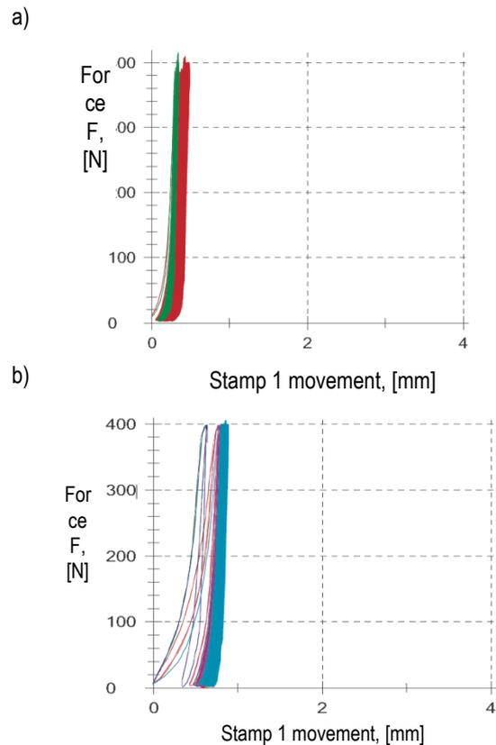
**Fig. 3.** Results of the test of cyclical loading of bridges a) without silicon insert, b) with the use of silicon insert
