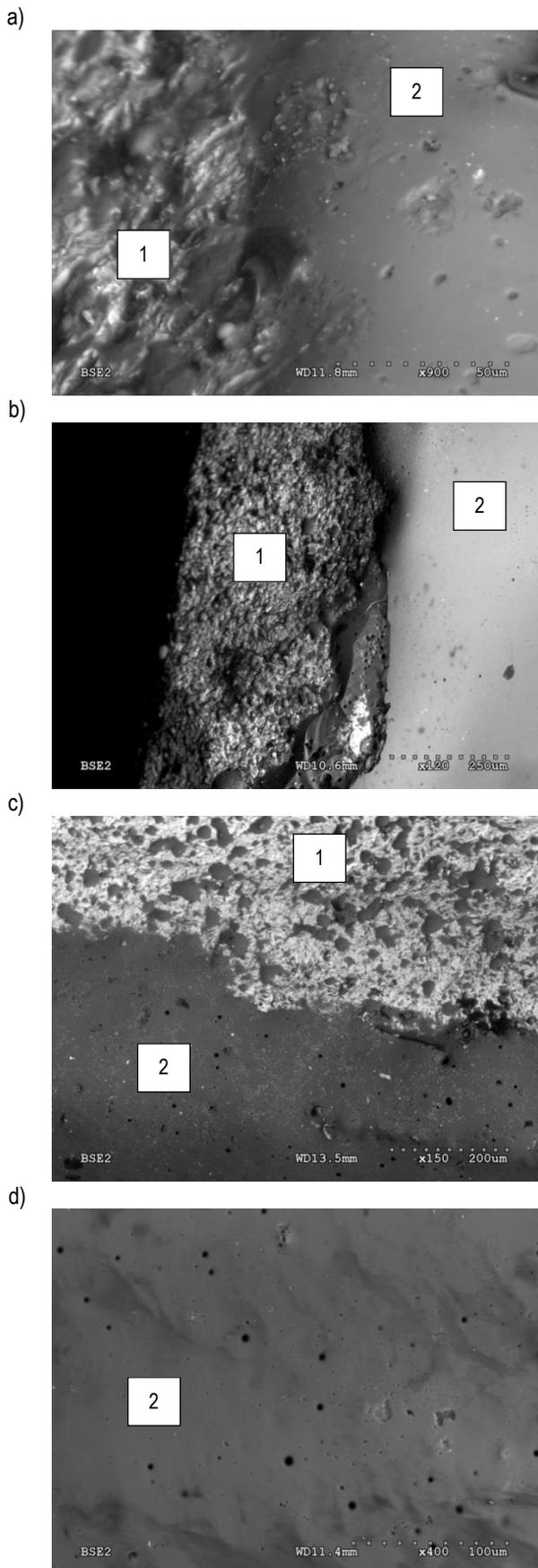
**Fig. 6.** Selected microphotographs of the surface of a porcelain bridge on a zirconia base: a)-c) pictures at the zirconia-porcelain interface, d) porous surface of the porcelain phase; 1 – zirconia phase, 2 – porcelain phase
