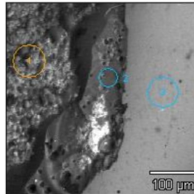
**Fig. 7.** Places of analysis of chemical composition – porcelain bridge on a zirconia base
