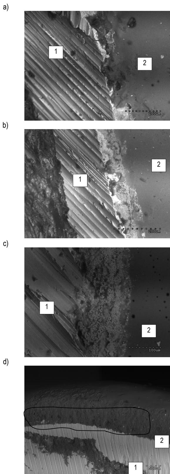
Fig. 4. Microphotographs of a porcelain bridge on a metal base: a) – c) view of the lateral surface on the metal-porcelain interface, d) view of the lateral surface; 1- metal, 2- porcelain
