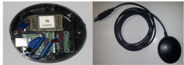
Fig. 2. On the left GPS Mouse Skytraq SJ-5210, on the right GNSSGM9 – picture of the receiver with USB-TTL interface in cover
