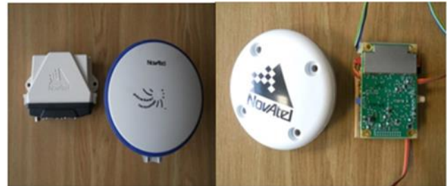
Fig. 3. On the right - picture of base station Novatel FlexPak G2-V2-L1 with Novatel GPS-701-GG antenna, on the left mobile receiver GNSS Novatel OEMV-1DF mounted on dedicated power board with ANT-35C1GA-TW-N antenna
